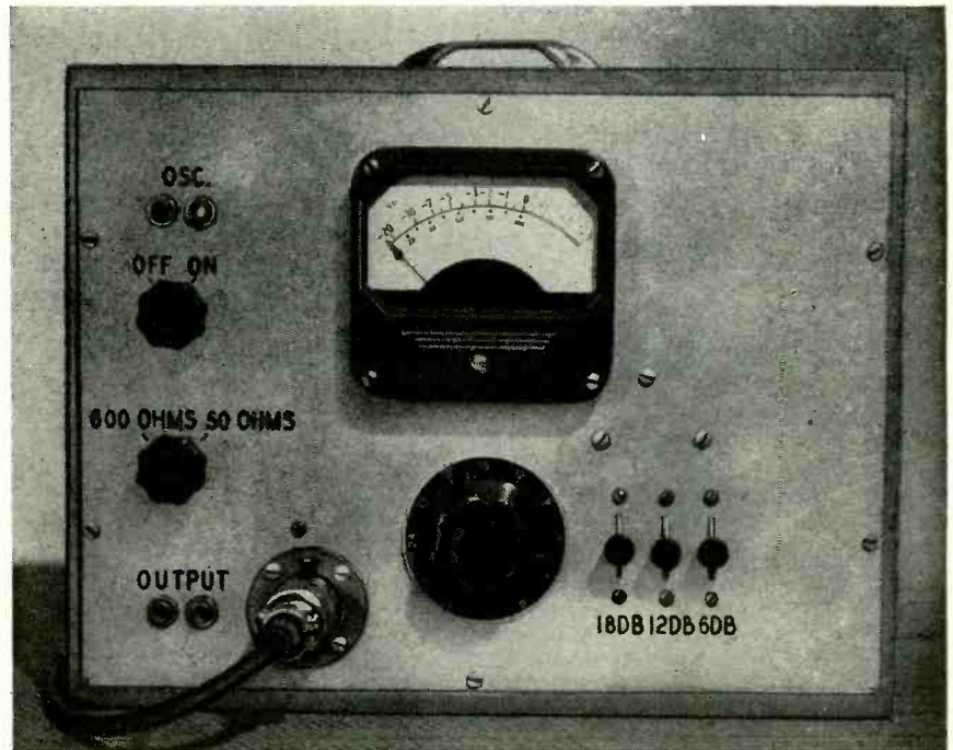
Photo shows front view of the transmission set. The cable connector parallels the output terminals to simplify feeding test signals to broadcast preamplifiers.
