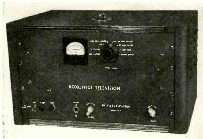
Fig. 9—The Boxoffice Picturecaster is a closed-circuit TV transmitter.
