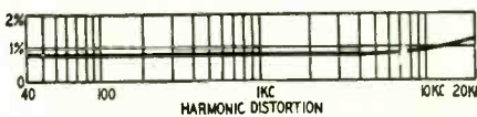
MEASURED WITH HEWLETT-PACKARD N/D METER 330-B (—65DB NOISE FIGURE. ALL MEASUREMENTS AT 5 WATTS)
